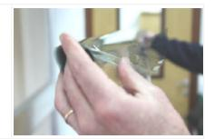
6. Firmly holding the film edge, gently throw the roll towards the ground. The release liner will peel itself off the film, and appear on the opposite side
